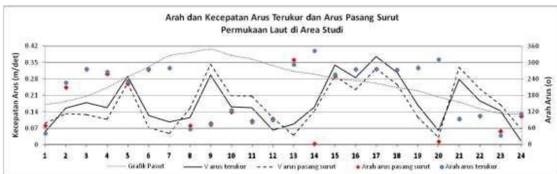
Figure 9. Graph of Direction and Speed of Measured Currents and Tidal Currents at Sea Level
